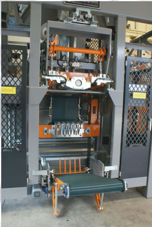
Press plates avoids over-compression
